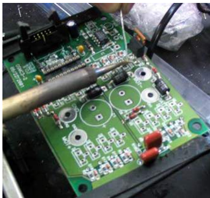
assembling the OSMC speed controller
