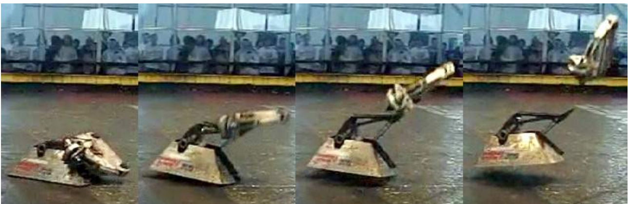
Launching with backward spin, due to a negative a_2
