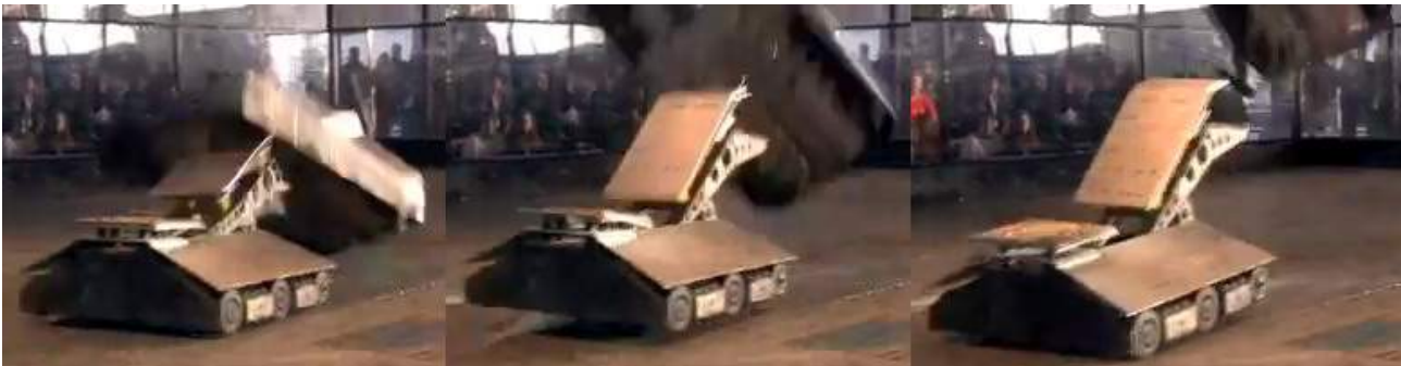
High range launch because of the almost neutral spin, due to a_2 close to zero
