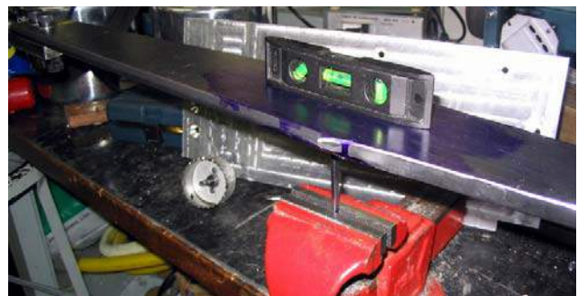
the center of gravity of each bar was found balancing them on the tip of a center punch
