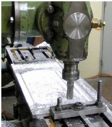
milling the top covers, to reduce weight
