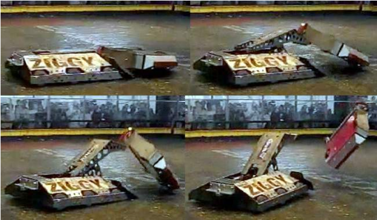
Launching with forward spin, due to the high a_2
