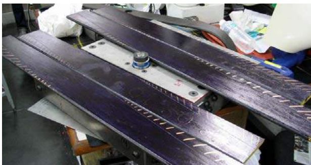
5160 steel bars for the weapon, before drilling and tempering
